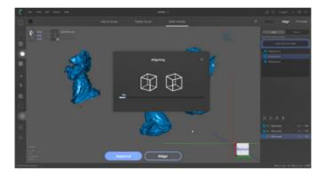
Now you can align the scanning results of different postures. First thing to do is make the models visible by picking up the scanning data, and click "align" to start automatic alignment. After finishing that, check whether the alignment is successful or not. If you're not satisfied with the result, click "manual" and start manual alignment.
