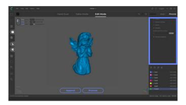
Once the alignment is done, click "process" to go through the automatic data processing. Before that, you can do some configuration about the processing.
