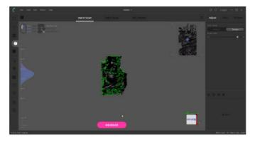
Click "preview" and there will be 10 seconds of countdown. During this period, you can adjust the brightness, the distance between the turntable and the scanner and your scanning angle.
