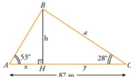
$$\text{En } \widehat{ABH}, \operatorname{tg} 53^\circ = \frac{h}{x} \rightarrow h = x \operatorname{tg} 53^\circ \quad \left. \begin{array}{l} x \operatorname{tg} 53^\circ = y \operatorname{tg} 28^\circ \\ 1,33x = 0,53y \end{array} \right\}$$
