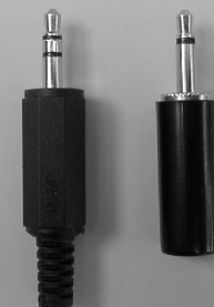
A mono plug (right) has one black band. A stereo plug (left) has two.
