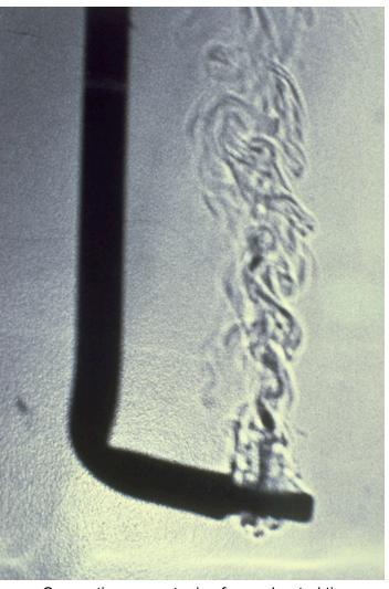
Convection currents rise from a heated tip immersed in a thin water tenk. The currents are made visible by the shadows they cas from a very bright, yet small-sized, lamp.
