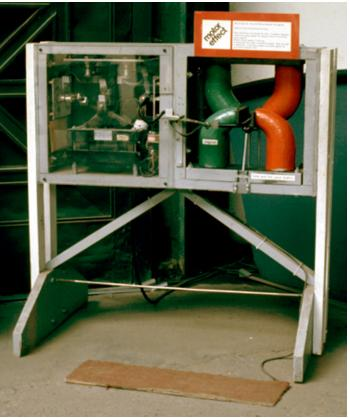
The Motor Effect Exhibit makes the wire in the magnet on the right jump when 200 amperes of current flows through it.
