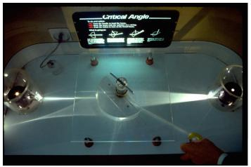
Light is refracted and reflected at Critical Angle.
