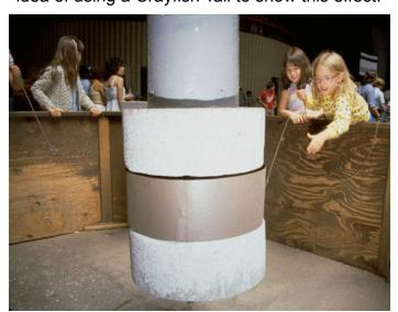
The giant 400-pound Resonant pendulum can only be given tiny tugs with weakly attached magnets and strings. A big swing can result if the tugs are timed with the swing of the pendulum.
